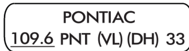
Sample VOR/DME NAVAID box with two SSVs
